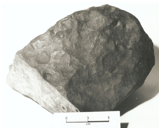
FIGURE 13 – Patos de Minas Meteorite (Areado Stream). On the left, part of the main mass, with a sub-rounded and flattened appearance, in accordance with Derby’s description. On the right, a slice of the meteorite polished and attacked with nital, exhibiting spots characteristic of hexahedrite-type meteorites. Because they have a lower nickel content, hexahedrites do not develop the Widmanstätten structure typical of octahedrites, which is also in agreement with Derby’s account. (credit: E. M. Zucolotto).
