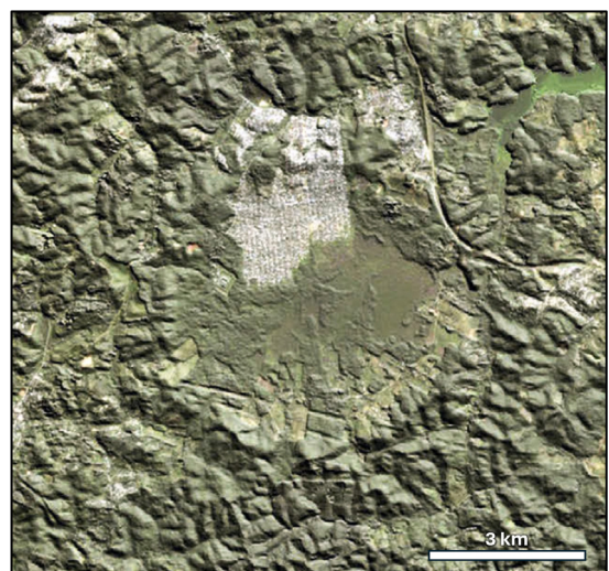
FIGURE 39 – Colônia. Composite image of the Sentinel-2 satellite, bands 2, 3, and 4 in RGB, superimposed on the TanDEM-X digital elevation model (GOTTWALD et al. 2020).
