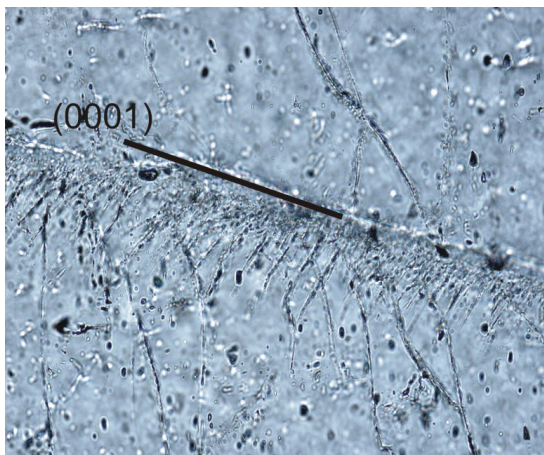
FIGURE 28 – Serra da Cangalha. Shock deformation microstructures (FF) in quartz grain from sandstone.
